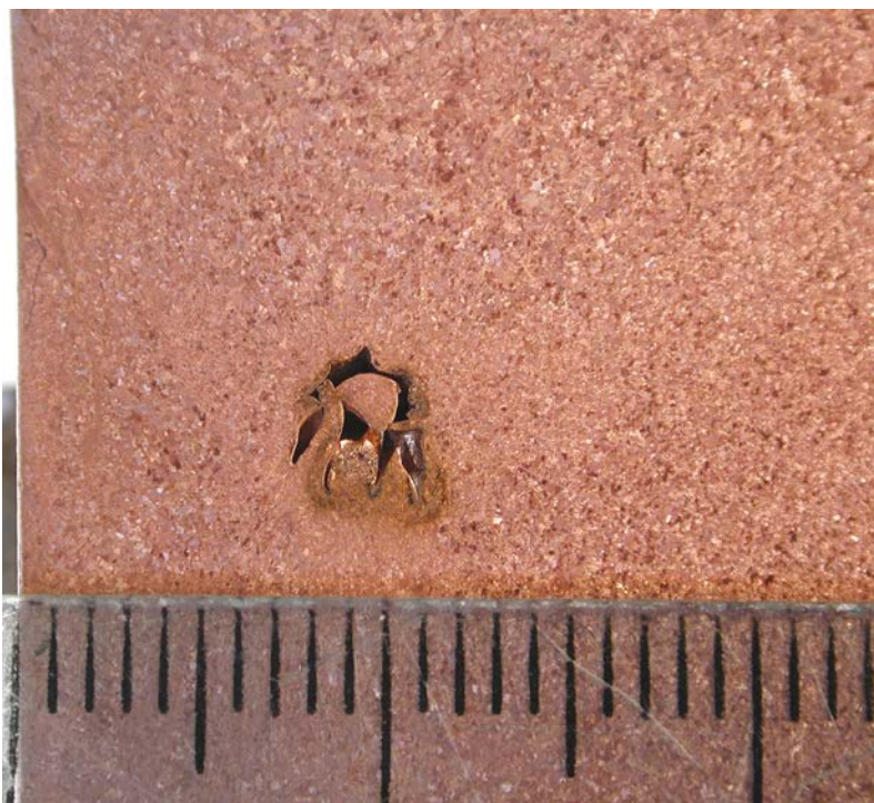
Figure 6-4. Macrospecimen of volumetric wormhole.
