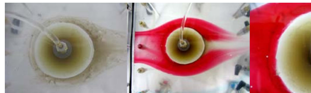
Figure 1. Overhead photographic images of an artificial fracture test with sodium montmorillonite against deionized water in a 1 mm aperture fracture at 456 h (far left image) and after dye injection (middle and far right images).
